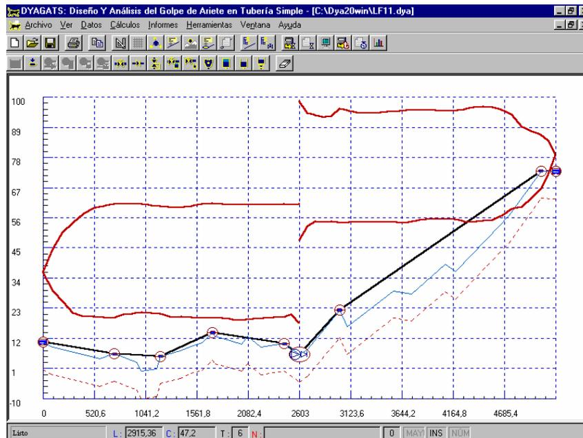
**Figure 8. Maximum and minimum envelopes after pump trip**
